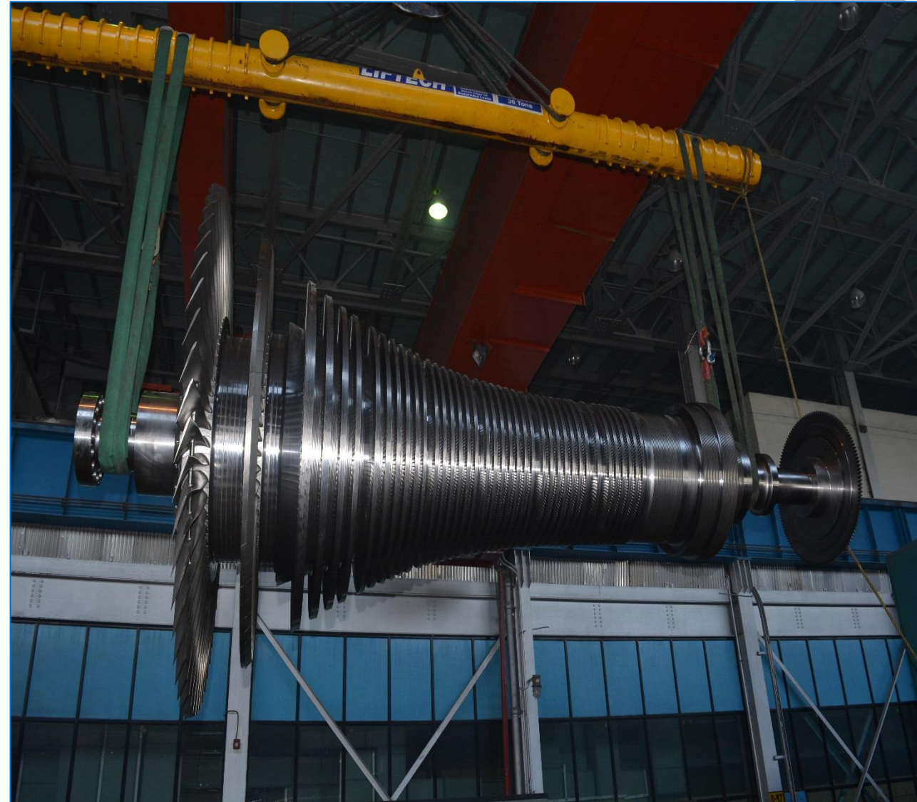
Unit-1 Proposed 77 MW Turbine Rotor
